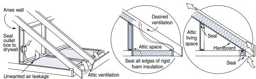
The attic knee wall is often underinsulated and leaky. Install adequate insulation and air seal around the living space for continuity in the building envelope when addressing the knee-wall door.
