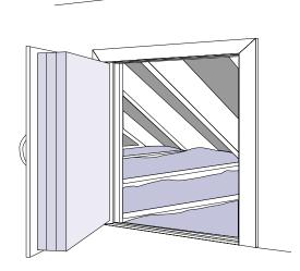
Add R-value to a knee-wall door by adhering rigid insulation boards (sandwiched together with construction adhesive and screws) to the back of the door. Pay special attention to the clearance between the insulation and the door frame and air sealing details.
