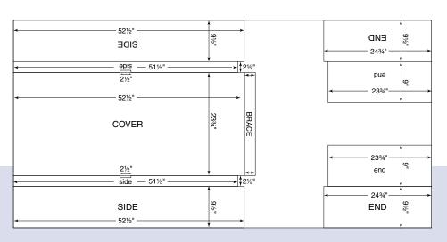
All pieces can be cut out of one 4'x8' sheet of rigid insulation. Use a table saw for smooth, accurate cuts.
